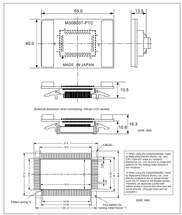
Figure 4.9 External dimensions of the M30800T-PTC
